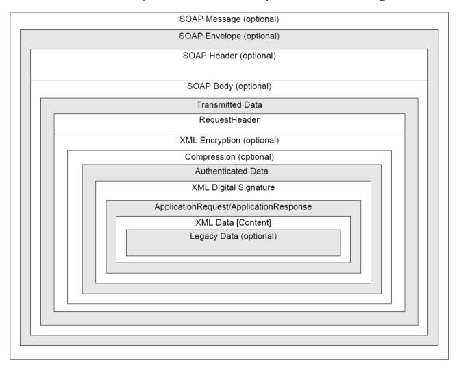
The RequestHeader (or ResponseHeader) wraps layers of compression, encryption and signing before the ApplicationRequest (or ApplicationResponse) can be accessed.
